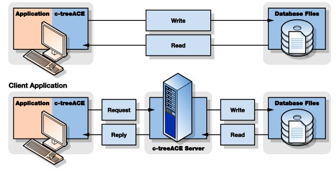
In the client/server architecture, database operations function in a client application program interfaced to a database server. The database server contains the "intelligence" needed to process requests from clients, interact with the relevant database files, wherever they are located, and respond to those requests.
