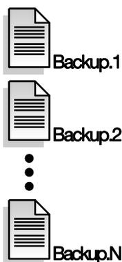
The Dynamic Dump backup feature defaults to breaking-up the backup file (stream file) into multiple physical files (segments). This gets around individual file size limits imposed by the host OS (e.g., 2GB for a typical Unix system). Each backup file segment defaults to 1GB. There is no limit on the number of backup files (segments) supported.
